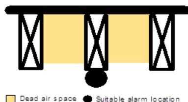
**Note:** The MFS does not recommend side wall installation.
