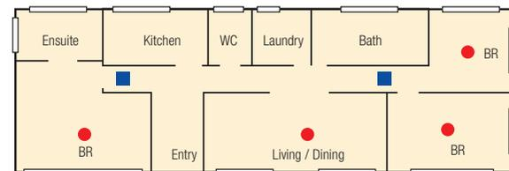
In passageways, the installation point should be at the end closest to the living area and certainly before the door of the first bedroom is reached so that when the alarm sounds, there will be sufficient time to allow evacuation through doors.
