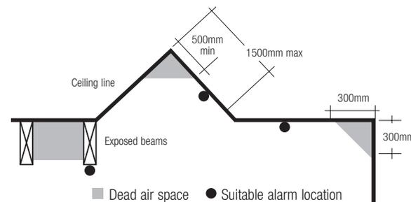
**Above:** Examples of the correct installation of smoke alarms with exposed beams, sloping ceilings and flat ceilings.
