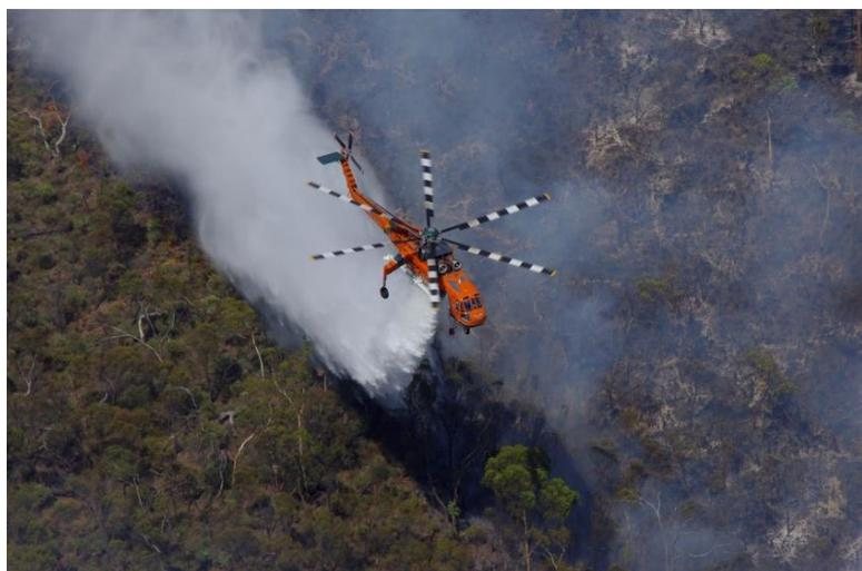
The Erickson Airplane S-64E dropping fire suppressant foam' on a fire edge to support ground firefighting resources.
